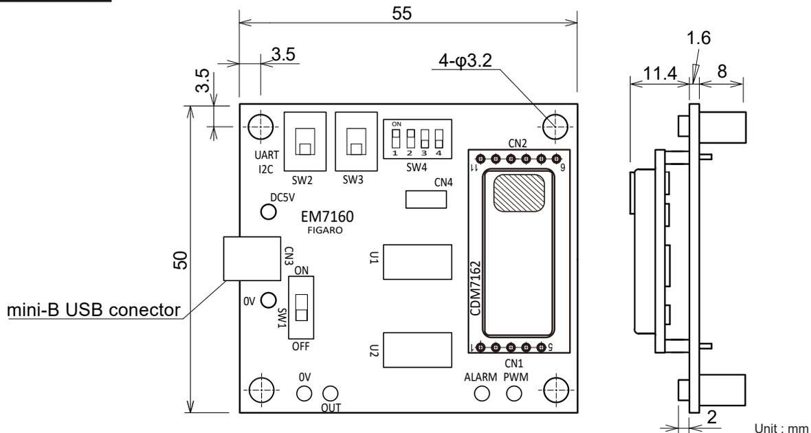
Note 1) Standard CDM7162 CO<sub>2</sub> sensor modules (without terminal pins) are available for additional purchase. To attach a standard CDM7162 to the evaluation module, terminal pins available in the marketplace should be soldered to the standard CDM7162.
