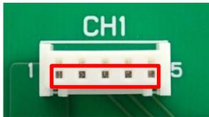
Insert the terminal of the gas sensor evaluation module into the larger hole of the connector for the module.
