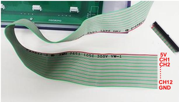
The signal wires coming out of the test chamber for gas sensor evaluation correspond to connector pins 1 to 50, starting with the red line.
