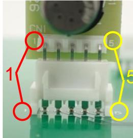
[Example of attachment of the test board for evaluation modules]
