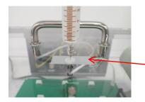
The adhesive tape is affixed to the top surface to prevent the "rubber for syringe insertion" from popping out. Replace it with a new adhesive tape as it ages.
