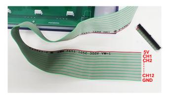
The signal wires coming out of the test chamber for gas sensor evaluation correspond to connector pins 1 to 50, starting with the red line.
