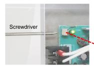
Turn clockwise (+)  $4.00V \rightarrow 5.50V$ Turn counterclockwise (-)  $5.50V \rightarrow 4.00V$
