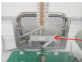
The adhesive tape is affixed to the top surface to prevent the "rubber for syringe insertion" from popping out. Replace it with a new adhesive tape as it ages.
