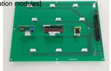
Match the pin number of the gas sensor evaluation module and the terminal number of the connector on the test board for evaluation modules, and insert it fully.
